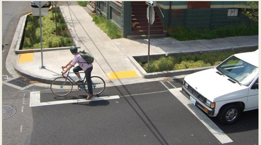
*Photo 25: Sample curb extension with bioretention facilities and expanded pedestrian ramps*
